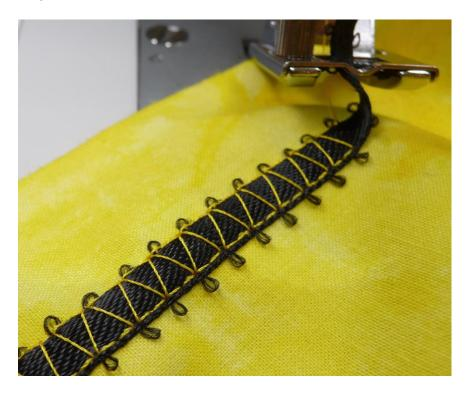
Guide ribbon into the foot and stitch along the sleeve hem, stopping near the end to trim excess ribbon. Overlap slightly, finish stitching, and then remove from machine. Treat raw end of ribbon with a slight amount of seam sealant.
