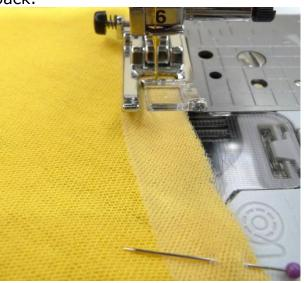
**Step 10**. Trim close to the stitching to remove excess stabilizer from the edge.
